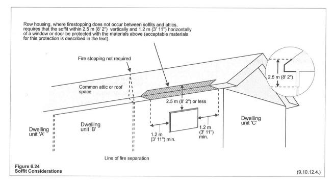
Per Section 9.10.12.4 of the National Building Code, to minimize the potential that fire will travel into an attic and across to another dwelling unit or across a fire separation as shown above, where an attic space spans more than 2 dwellings the soffits must be protected above any door or window where sprinklers or attic fire blocking are not provided.
